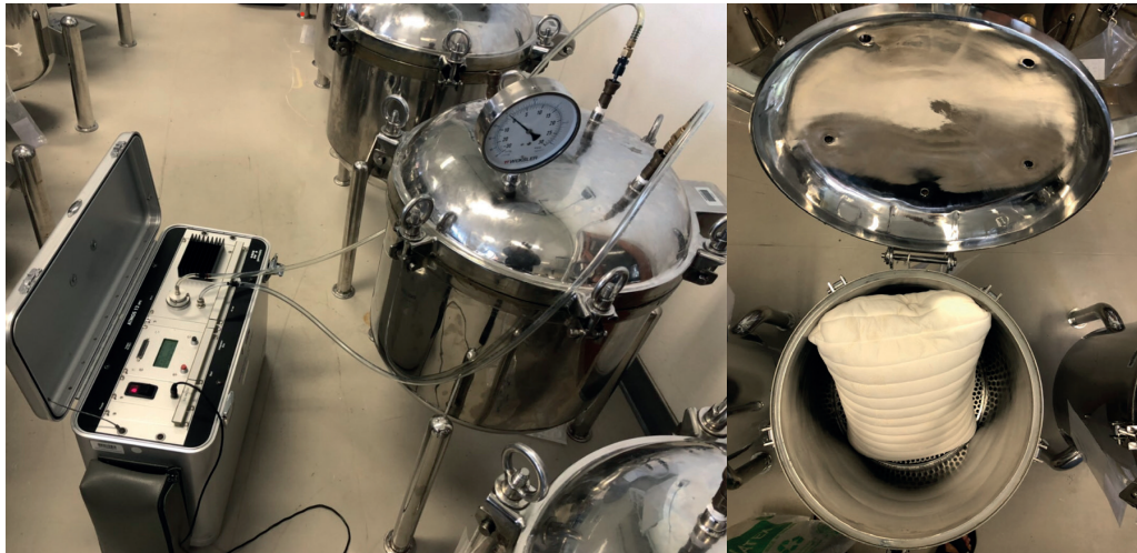
Figure 1 The equipment set up to measure radon concentration and radon exhalation rate, which the natural rubber latex pillows were placed inside the closed-chamber with connected to the pulse counting ionization chamber (ATMOS 12 DPX).
